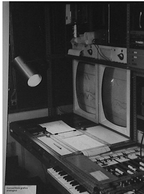
Figure 4. The Analog Graphic Converter developed by Fernando von Reichenbach at CLAEM during the late 60s.
